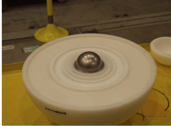
Figure 3.3: The BeRP ball was developed by Los Alamos National Laboratory in 1980. The acronym stands for beryllium-reflected plutonium, but that is an anachronism. Today, the Pu sphere is surrounded by polyethylene shells which serve to scatter neutrons and increase the k_{eff} of the source. It is often used as a source to verify Monte Carlo transport code as well as an inspection object for treaty verification.
