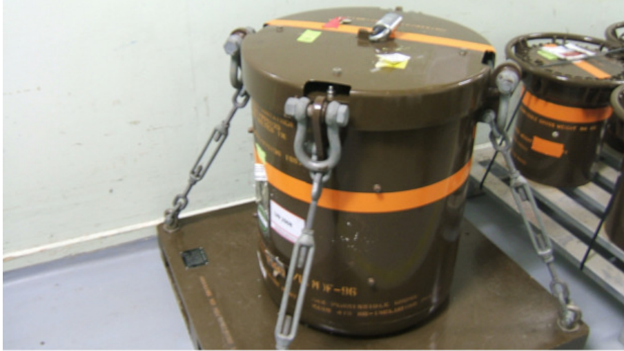
Figure 1.8: An example storage container for a warhead.
