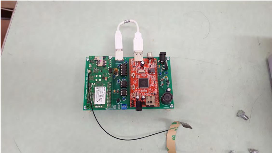
Figure 2.3: A fully assembled printed circuit board for a custom sensor. The red board is the OLinuXino and the green board on the left is the cell modem with a flexible antenna. Through hole components were chosen for easy soldering.
