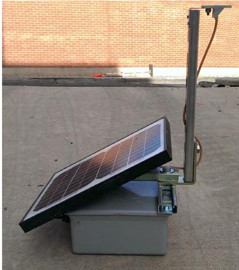
Figure 2.5: A photo of a complete custom irradiance sensor as it undergoes testing outside. The photodiode sensor can be seen mounted in the upper right of the image connected via a coax cable to the circuitry inside the box.
