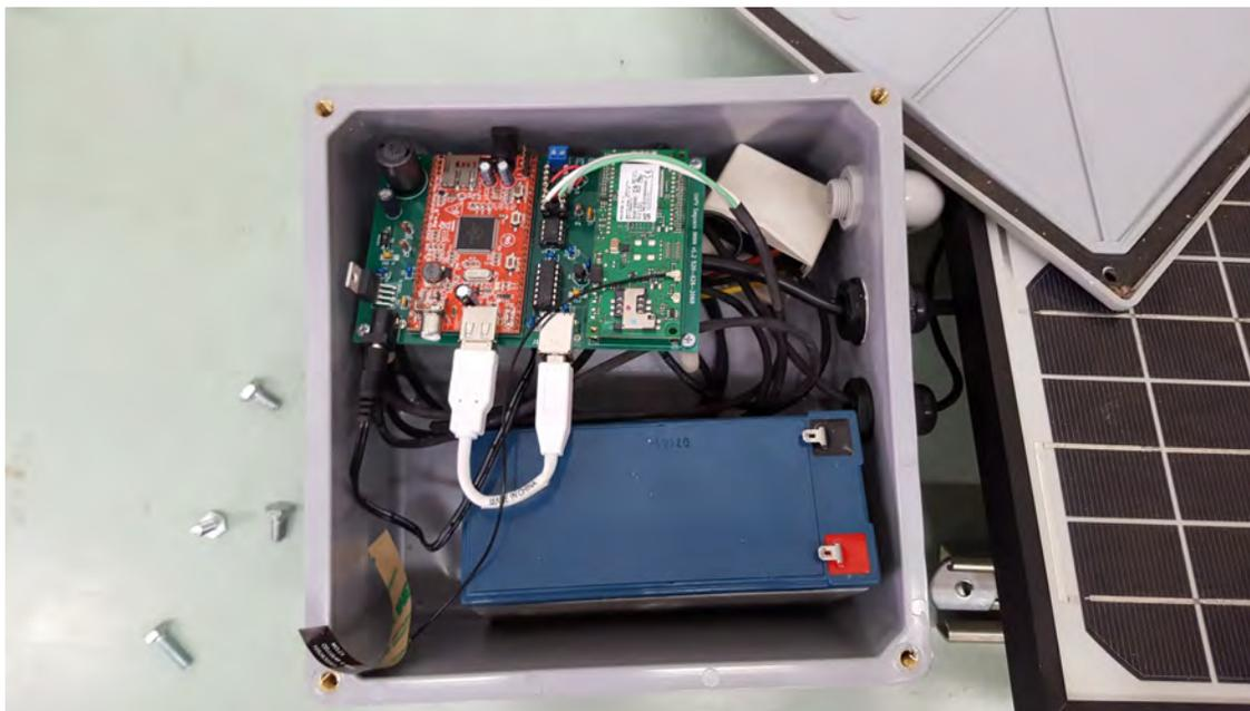
Figure 2.4: A photo of the interior of the sensor enclosure. The air vent and waterproof cable nipples are visible on the right side of the box. The 6Ah 12V motorcycle battery is shown near the bottom.
