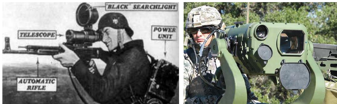
Figure 1.2. Military infrared detecting devices: past and present. German infrared night-vision devices, ZG1229 (left) and 3rd Gen eLRAS3 FLIR system (right). The improvements compared to the past are following: 1) switch from active to passive system to prevent users from exposing their positions, 2) detect both long and medium wavelengths (both body temperature and heat from equipment), 3) dramatic increase in resolution and detection range [4, 5].
