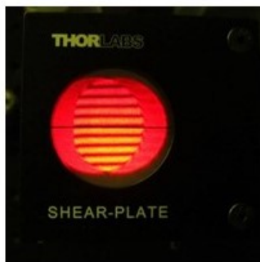
Figure 6.18: Shear plate interferometer showing straight line fringes indicating the light reflecting off of the OAP is collimated and free of aberrations (Newman, 2013).
