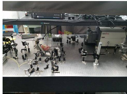
(c) The lab bench hosting the Zygo interferometer and high contrast imaging setup
