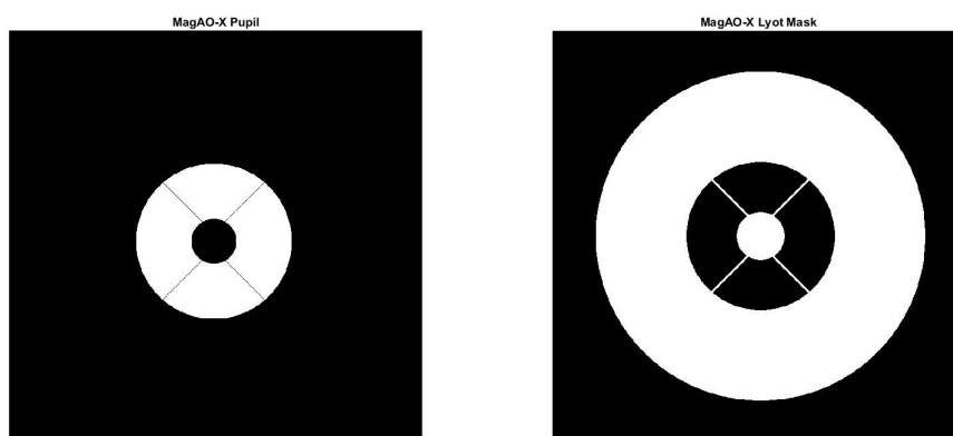
Figure 6.2: MagAO-X masks: Entrance pupil mask (left) and the reflective Lyot stop used for the following LOWFS simulations (right)
