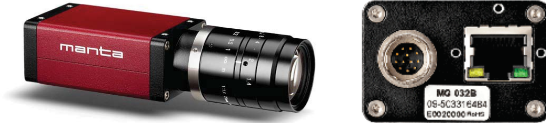
Figure 3.45: Cat's eye camera, AVT Manta G419B-NIR.
