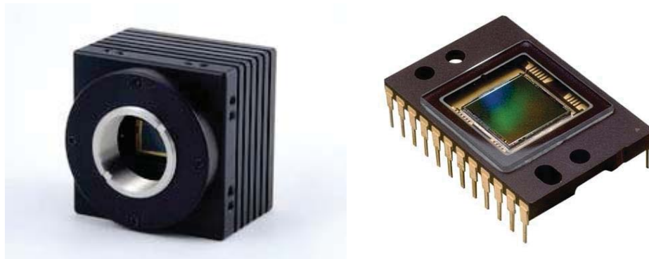
Figure 3.44: Camera system used by the 4D pixelated sensor. (Left) MMV-1010. (Right) KAI-1010.
