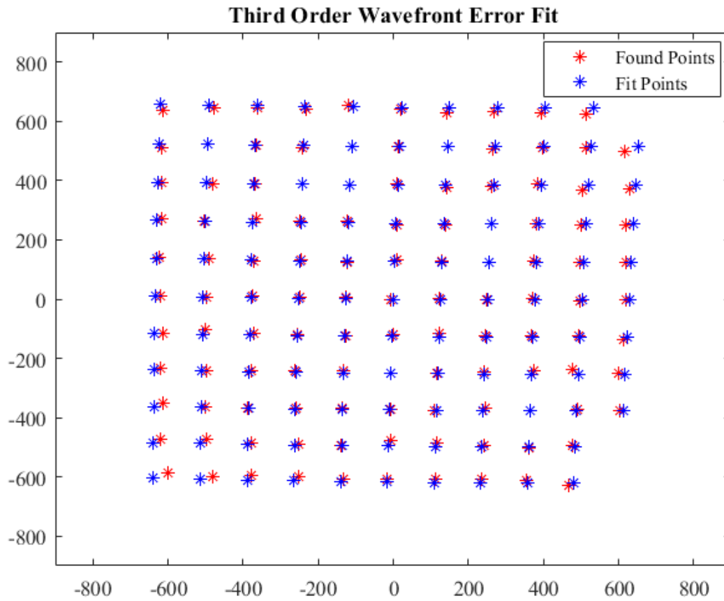
Figure 4- 23: 3 rd order wavefront error point fitting. The 3 rd order fit is successful at fitting most field points but deviates at the very edge of the field. The mild barrel distortion remains uncaptured in the fitting at second order.
