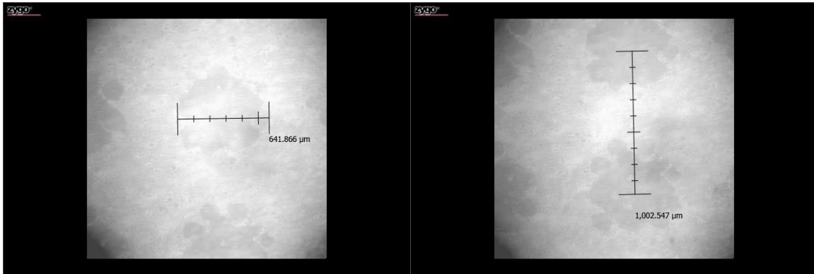
Figure 2- 4: The printed dot diameter and shape (left) is approximately 0.642 mm and the nominal center to center dot spacing (right) is approximately 1 mm.
