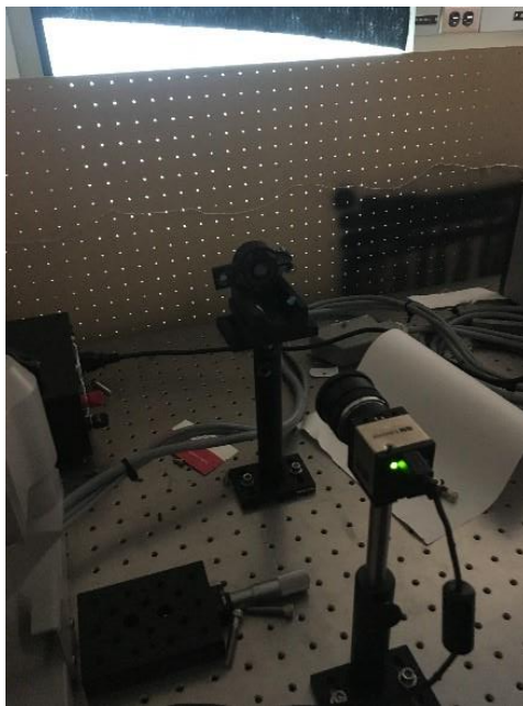
Figure B-1: Pegboard experimental setup. Note that this section used a cardboard aperture with 1" holes placed over the diffuse light source in place of the pegboard shown in the image. Spot patterns on the back of CFB are captured with a RGB Point Grey camera for processing.
