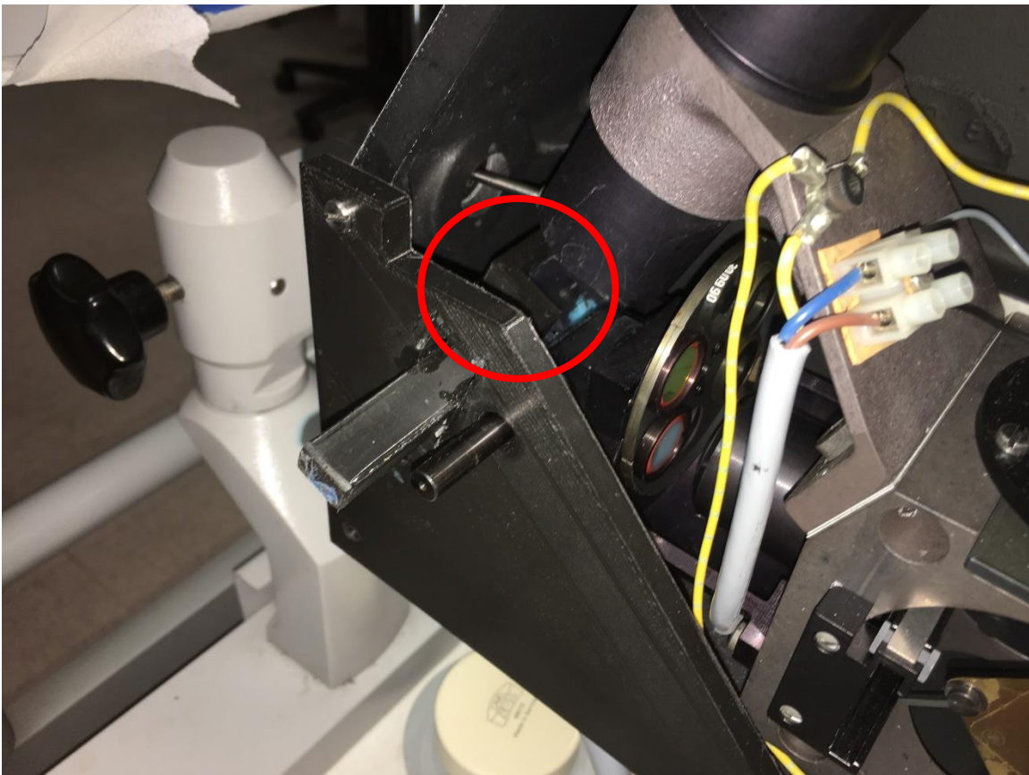
Figure 2- 5: 3D printed cover and grid target holder. The grid target, fixed to a glass plate, is located inside the red circle of the image and placed conjugate to the retina.
