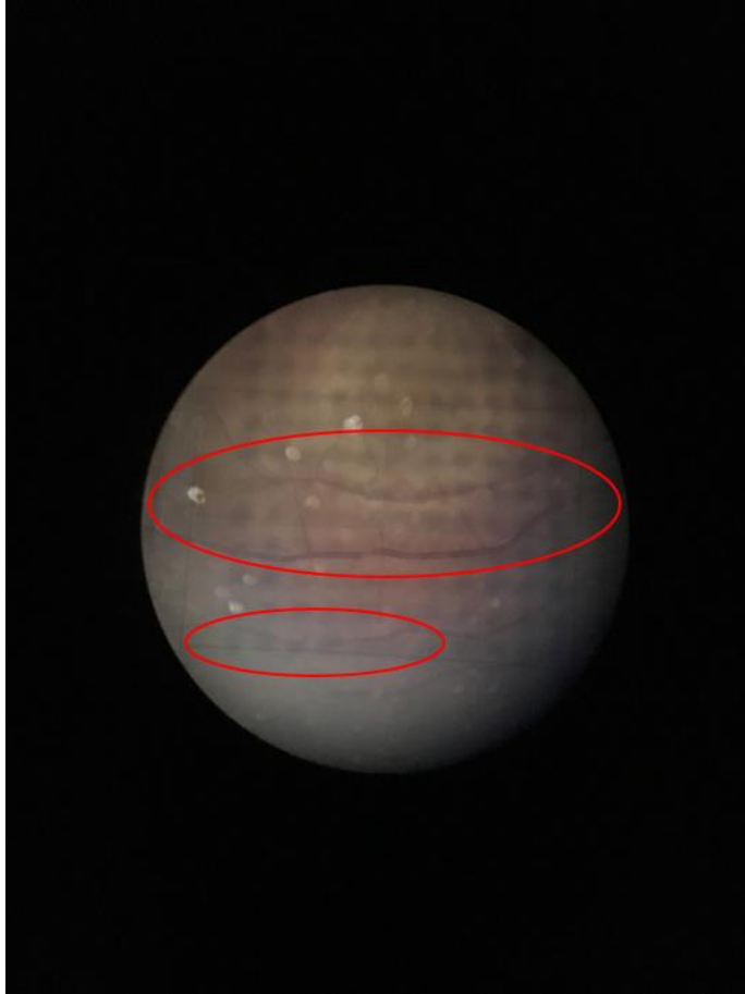
Figure 5- 7: Target dot deformation around blood vessels. Dots appears to move with the meander of blood vessels in the red circled areas. Local curvature departures are the proposed cause.
