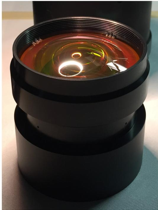
Figure 24: Element 1 tack bonded into Forward Lens Cell
