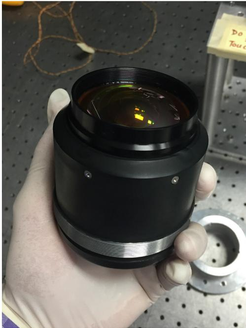
Figure 27: Objective Lens Assembly - Front
