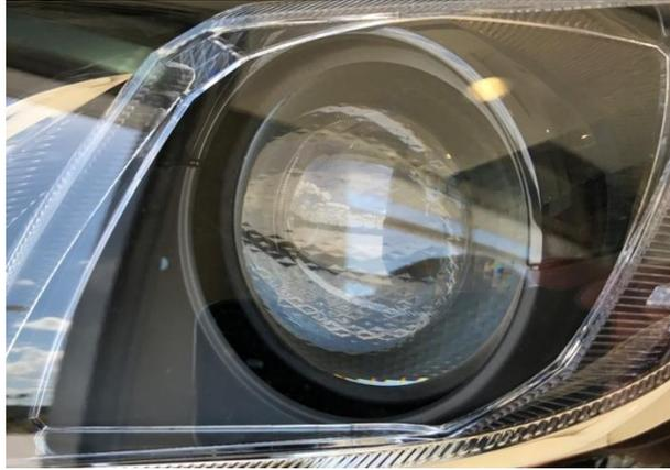
Figure 1-1. Projector-type headlamp lens
