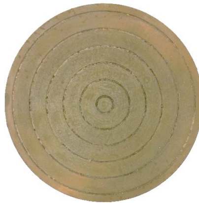
Figure 22 Grinding tool with Radius of Curvature of 1000 m used for conditioning other grinding tools.
