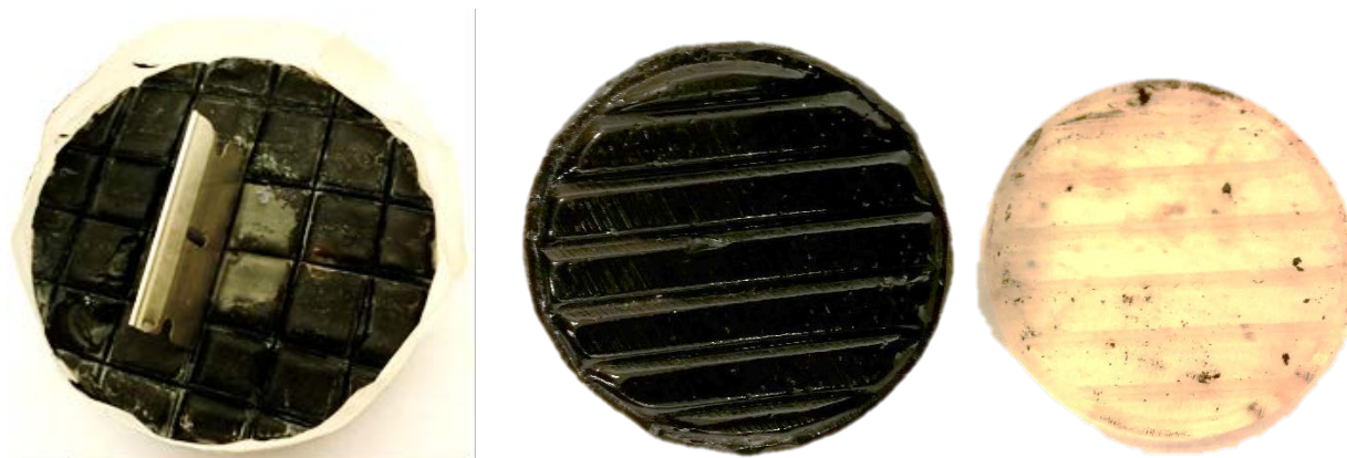
Figure 19 Pressing pitch (left), pressed pitch with 3D printed tool (center) and tool (right).
