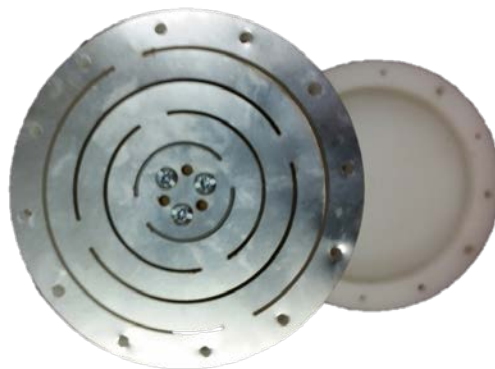
Figure 6 Aluminum flexures mounted between rigid 3D printed part.
