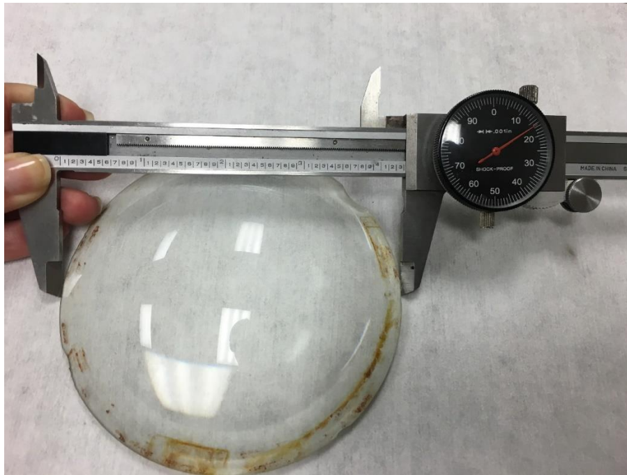
Figure 11: Thickness Measurement of a Lens in the Lab
