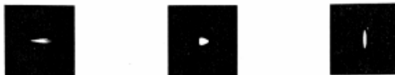
Figure 22: Example Astigmatic Lines. Tangential focus (left), Medial Focus (center), Sagittal Focus (right) (Parks, 1980).
