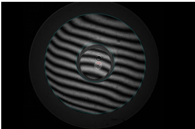
Figure 9: Final Interferogram of OPTI 597B Primary Mirror
