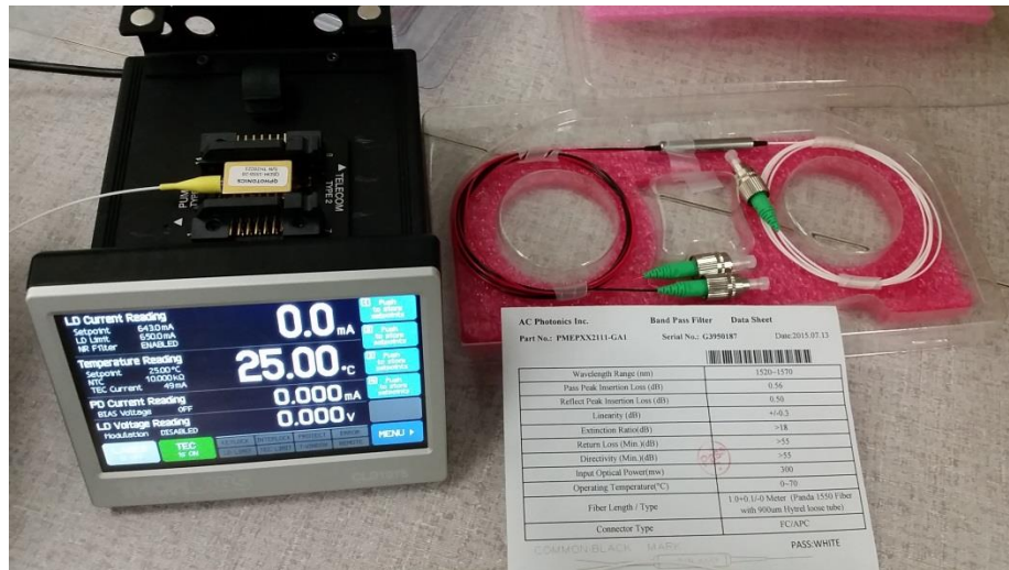
Figure 6.2: Broadband source laser diode, controller, and bandpass filter
