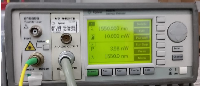
Figure 6.1: Narrow-linewidth, fiber-coupled laser source
