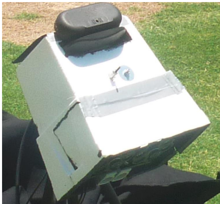
Figure 21: Mounted camera box, with fan and cameras inside.
