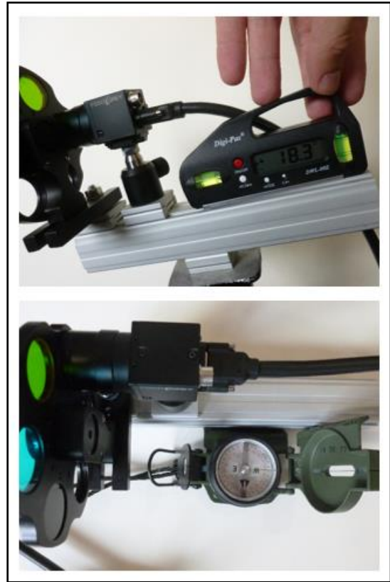
Figure 31: Measuring the zenith and azimuth angles with respect to the optical rail.
