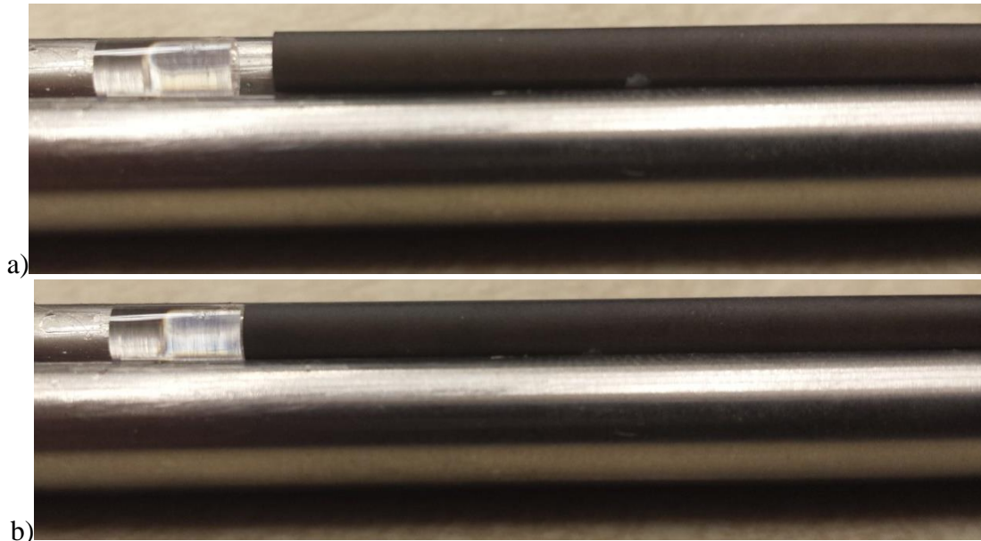
Figure 3.13: Placement of the GRIN lens and GRIN rod a) prior to placing epoxy droplet b) after applying epoxy droplet
