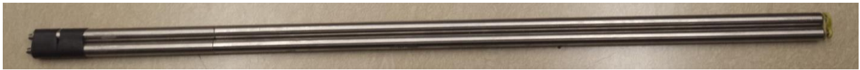
Figure 3.12: V-groove assembly created out of 10 inch and 3 inch cage rod components from ThorLabs
