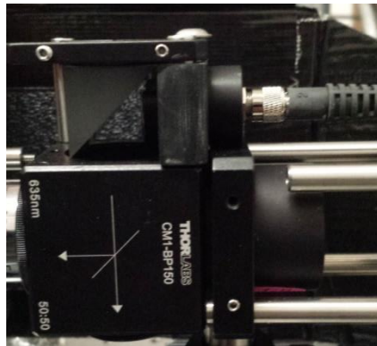
Figure 3.16: Placement of the illumination fiber and optics into the pellicle cube.
