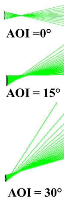
Figure 1.12. Simulated RPC EDC20 lenslet performance for 0°, 15°, and 30° AOI. Off-axis performance is dominated by coma and astigmatism.
