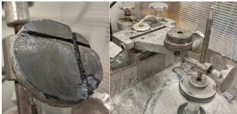
Figure 5.13: Polishing lap (left) and polishing process on Strasbaugh (right) with 1933g lead weight on the polishing arm.
