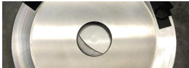
Figure 5.23: Guide ring over the two-fiducial fixture with a finished fiducial visible on the glass.
