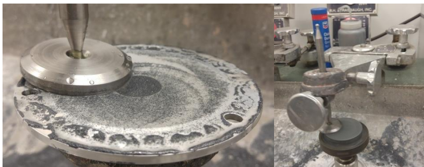
Figure 5.6: Close up view of a guide ring and grinding tool in the coarse grinding phase (left) and a broader view of the grinding and polishing Strausbaugh machine grinding on a conditioning plate.
