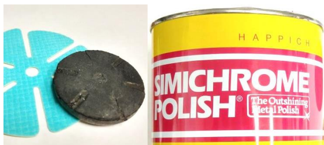
Figure 5.8: Polishing tool and polish for polishing conditioning plate and guide ring.
