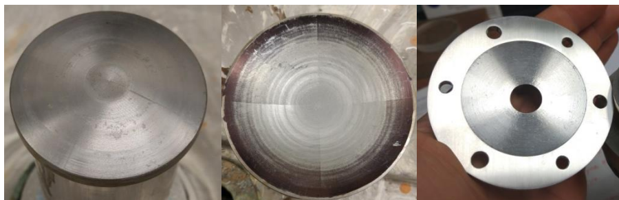
Figure 5.5: Machined surface of the steel grinding tool (left), steel conditioning plate after some coarse grinding (center), and aluminum guide ring after machining (right).
