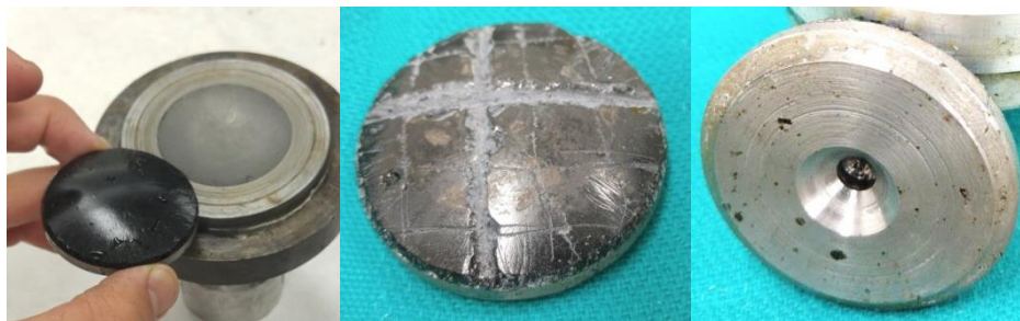
Figure 5.7: Polishing tool pressed out on conditioning plate (left), polishing tool with channels cut and broken in (center), and ball socket machine interface (right).
