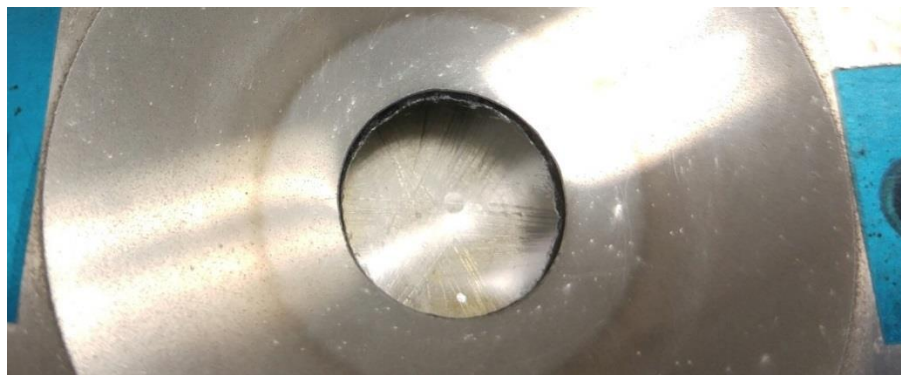
Figure 1.14: Phase fiducial on an optical flat surrounded by fabrication guide ring. Radius = 80 mm, CC and \varnothing = 2 mm
