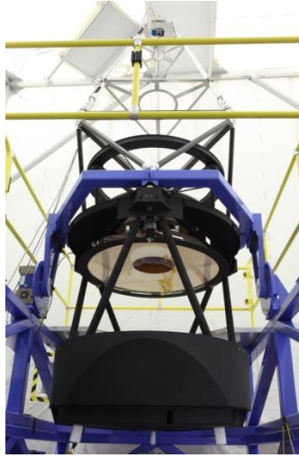
Figure 2.1: HET WFC in assembly and testing mount with interferometer mounted in tower above system.
