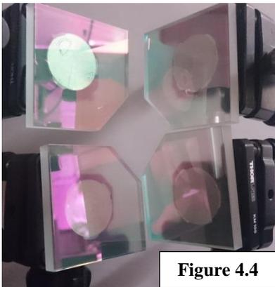
The four fold mirrors were selected using modified Thorlabs BBSQ2-E03 2"x2" square dielectric broadband coated mirrors (750-1100nm). They have a reflectance of >99.5% at 45° angle of incidence. The mirrors were modified using a diamond cutting wheel to cut
