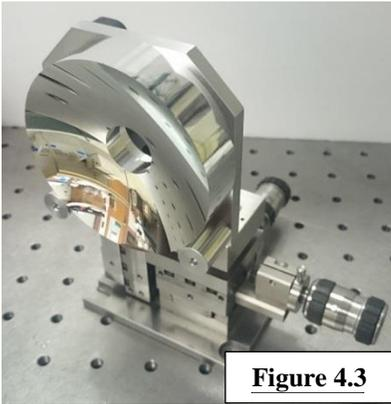
The focusing mirror was chosen to have a focal length of 35mm with an external diameter of 78mm and an internal hole aperture of 20mm. It was manufactured as a parabola (-1 conic constant) using an aluminum substrate with an enhanced aluminum coating centered at 795nm,
