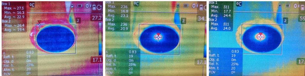
**Figure 5.6** Pump spot temperature experience in thin disk.
