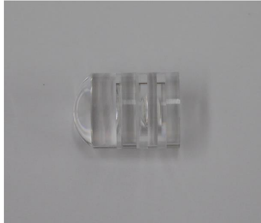
Figure 4.23 Microscope objective after all the lens elements are assembled together.
