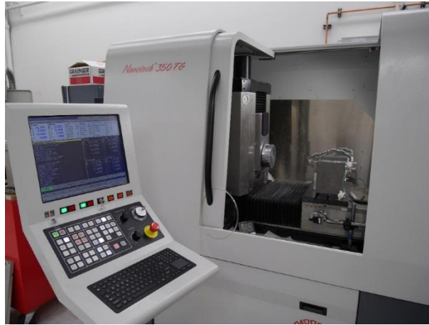
Figure 1.1 Four-axis diamond turning machine 350 FG from Moore Nanotechnology Systems.
