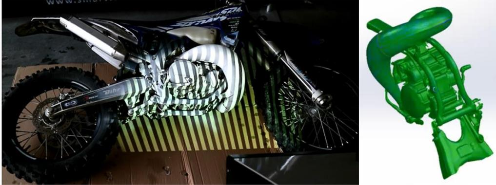
Figure 3.15: (Left) 3D imaging of motorcycle parts with structured light method. (Right) Rendered 3D model after manual touch up [36].
