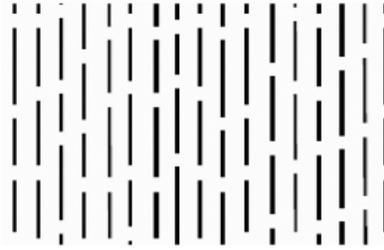
Figure 3.8: An example of stripe indexing with segmented line pattern [23].
