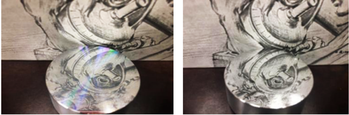
Figure 24 Visual appearance of the Al6061 sample before (left) and after (right) the smoothing process.
