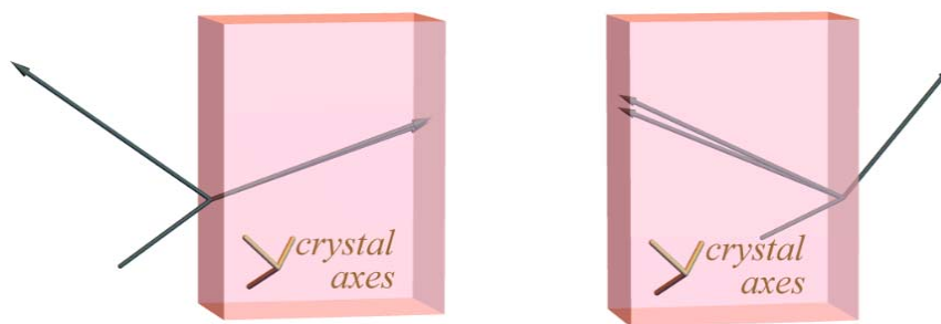
Figure 2.16 External (left) and internal (right) reflection and refraction of biaxial interface.
