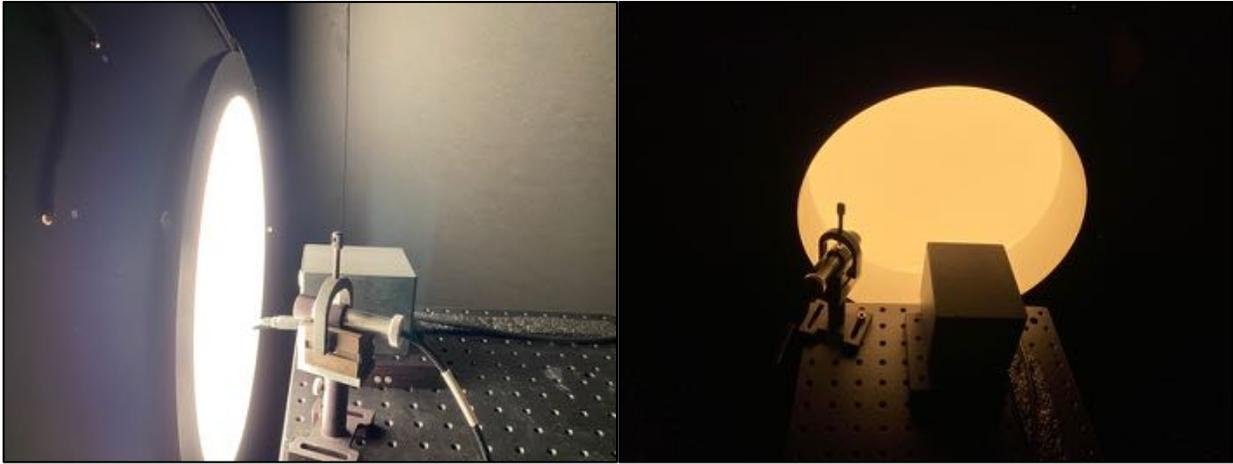
*Fig. 22: ASD spectroradiometer and micro-spectrometer set up in front of the SIS to view same target area for radiometric calibration.*
