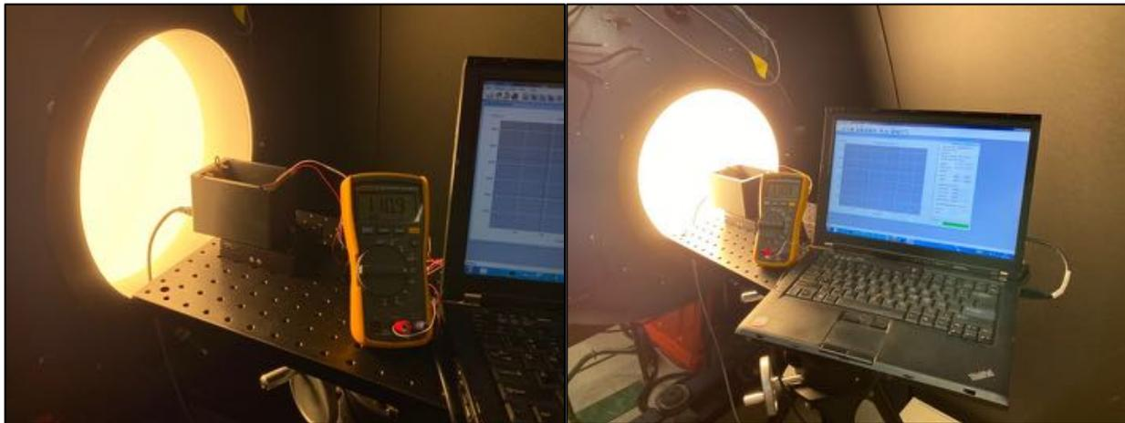
*Fig. 27: Testing setup for measuring the responsivity dependence on temperature.*
