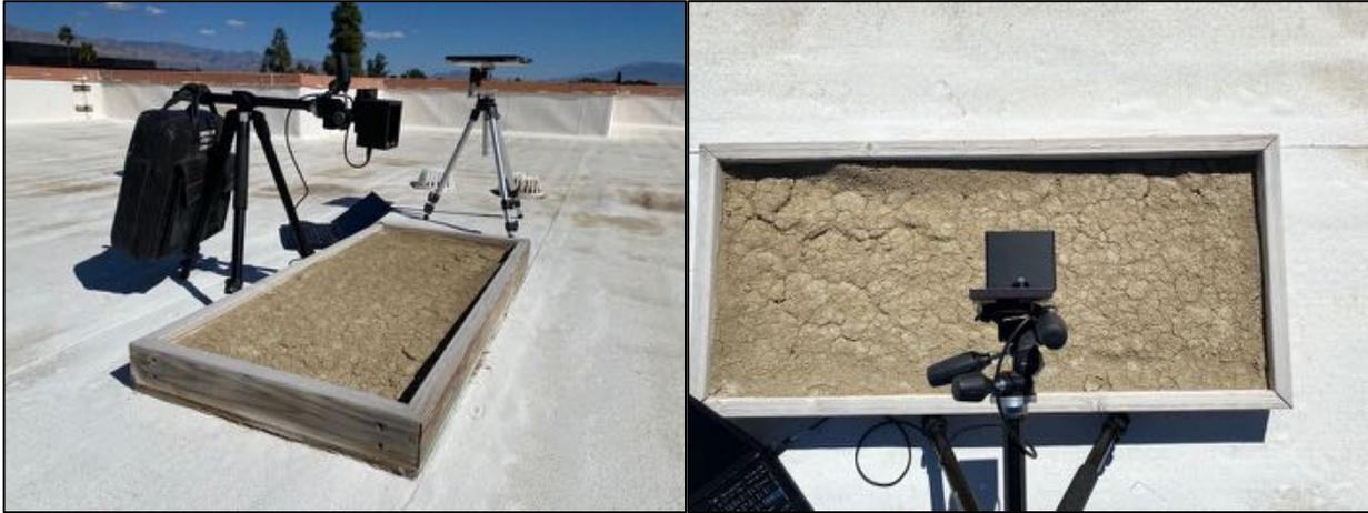
*Fig. 25: Setup for optimal integration time characterization. Measurements are made of the Spectralon panel and RRV soil. The instrument is positioned such that only the surface of interest is within the FOV.*
