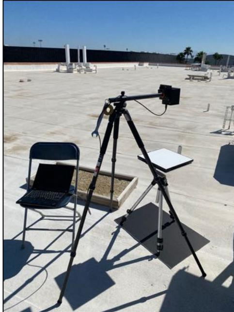
*Fig. 23: Setup for making measurements with panels. The setup shown here is for measuring the Spectralon panel. The same setup is used to measure the 48 % panel.*
