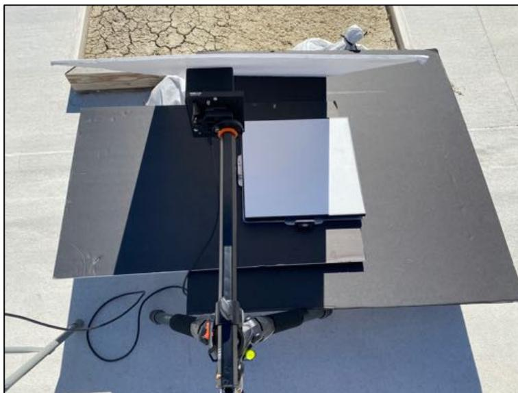
*Fig. 24: FOV test setup. Spectrometer is traversed from the edge of the black panel to Spectralon panel in both x direction and y direction. Note: panel resting on spectrometer provides shade to the plastic and electronics during downtime and is not present during testing.*
