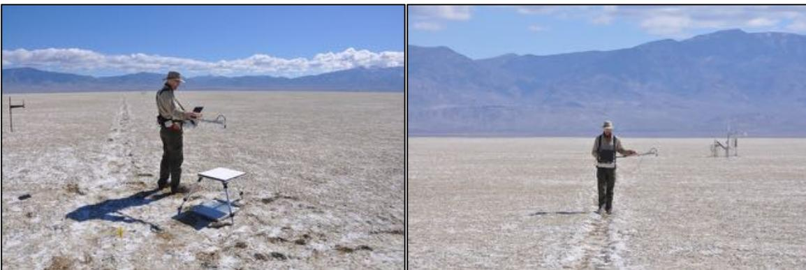
Fig. 2: Remote Sensing Group member recording a reference panel measurement with ASD (left) and walking Railroad Valley with an ASD and recording ground measurements (right).
