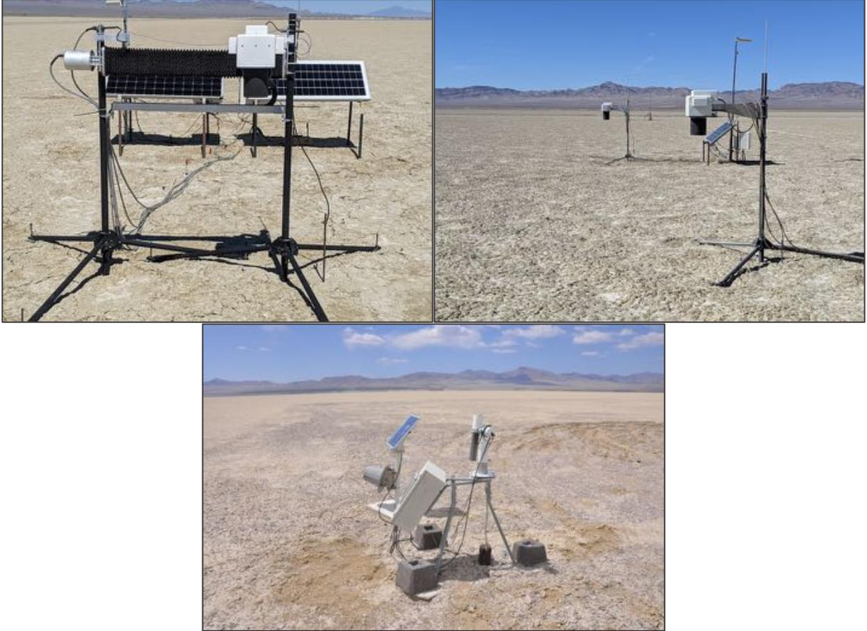
Fig. 5: GVR equipped with linear motion (Top Right), stationary GVRs (Top Left), Cimel sun photometer (Bottom).
