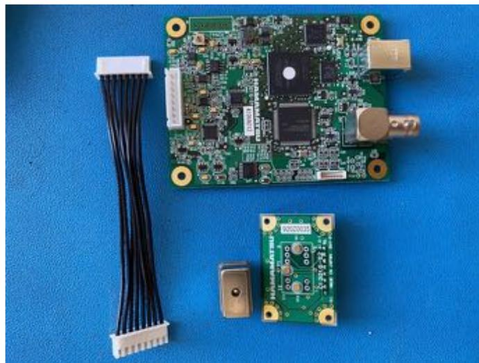
Fig. 13: Components in the C13016 evaluation, including the sensor board, connection cable, and evaluation board. Also shown is the micro-spectrometer.
