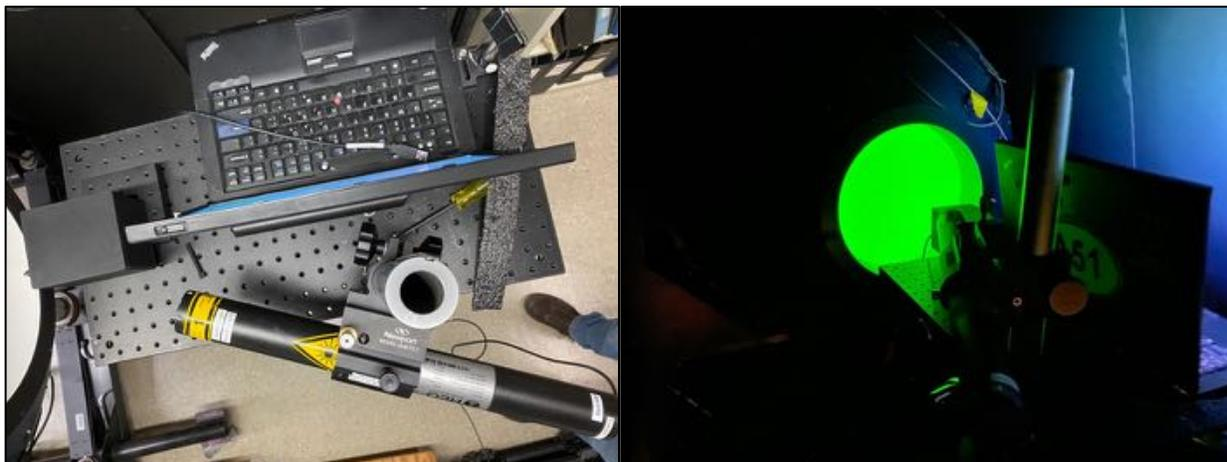
*Fig. 29: Laboratory setup for spectral characterization. Left picture is a top view of the setup, spectrometer is centered in the sphere aperture and the laser is positioned to send an unobstructed beam into the SIS. Right picture shows the green laser illuminating sphere. The red laser is substituted for the green laser during the 633 nm measurement.*
