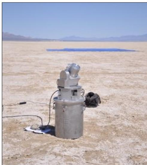
*Fig. 3: Automated solar radiometer used to take atmospheric measurements.*
