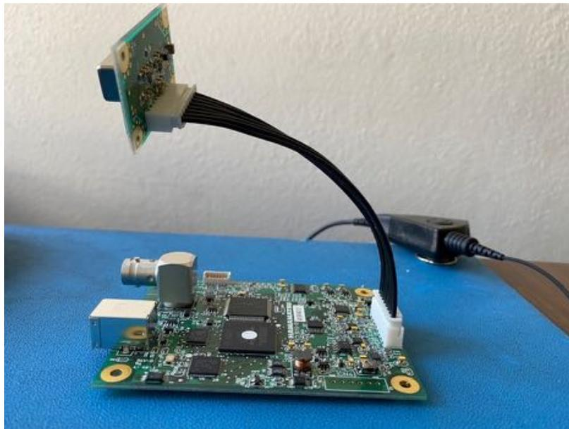
*Fig. 14: Assembled evaluation circuit.*
