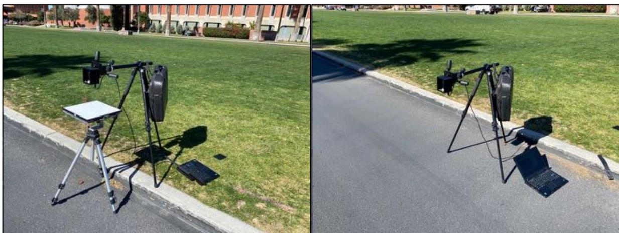
*Fig. 30: The setup for measuring the surface reflectance of asphalt. The same setup is used for other surface measurements.*
