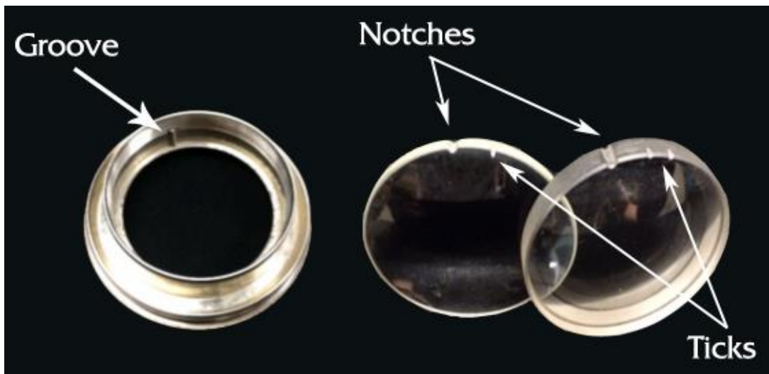
Figure 3. Clocked refracting telescope objective composed of a brass barrel with a groove and notched lenses
