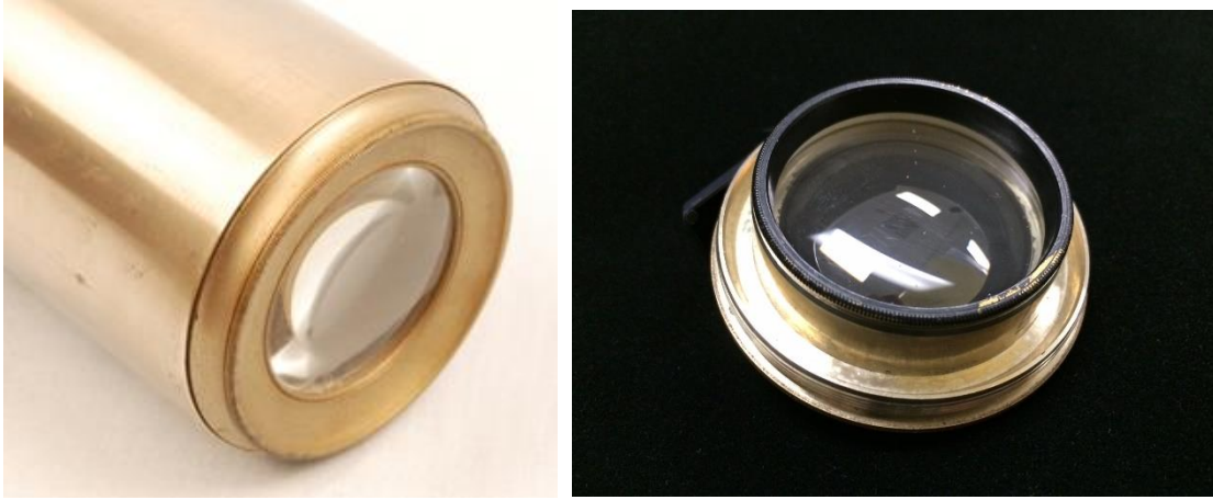
Figure 5. T59 objective mounted in the telescope barrel and alone in its cell
