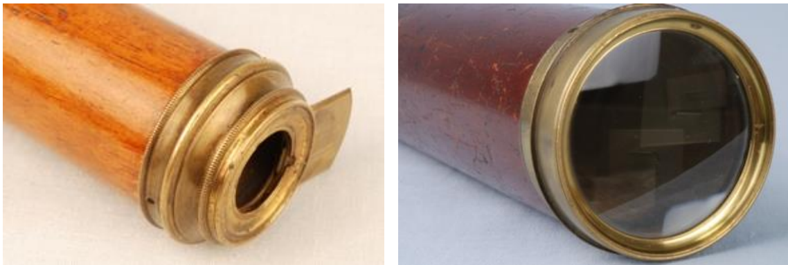
Figure 1. Comparison of a pre-achromat refracting telescope objective (left) and an achromat telescope objective (right)
