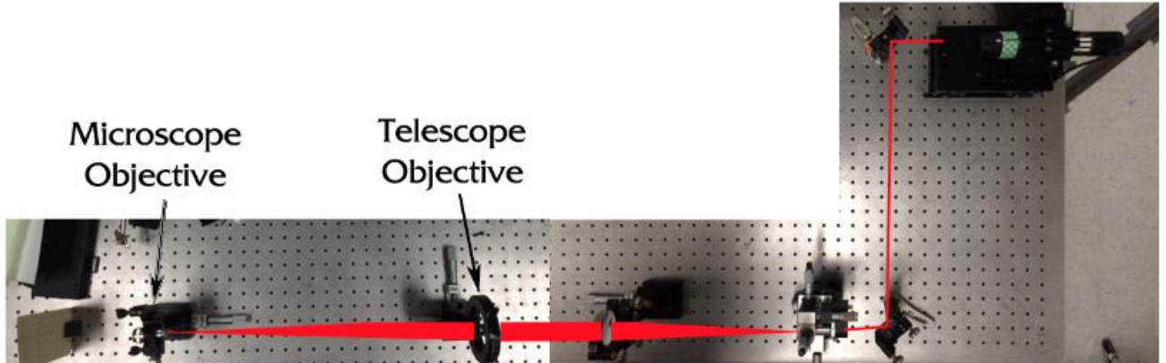
Figure 23. Lab bench setup for the simulated star test
