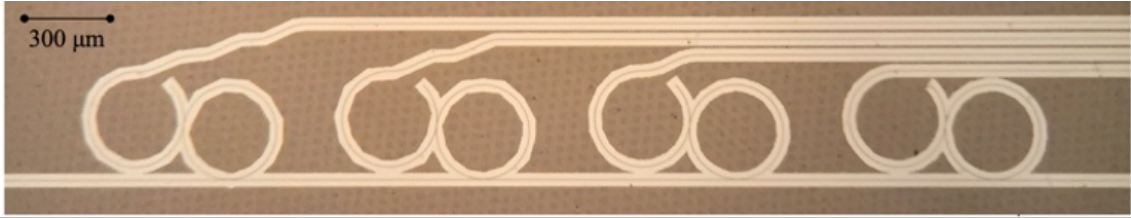
Figure 4.1: Si 3 N 4 chip design with microring resonators.
