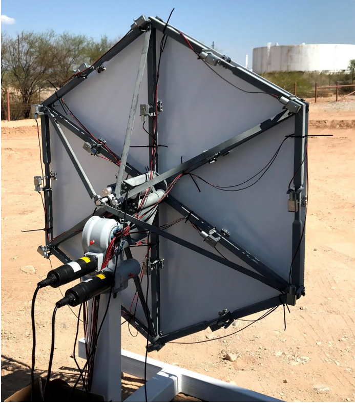
Figure 4.4: Back view of prototype heliostat structure. The altazimuth tracking mechanism is visible along with the 18 adjustable pads and the 3 linear actuators, each attached to a pair of struts.
