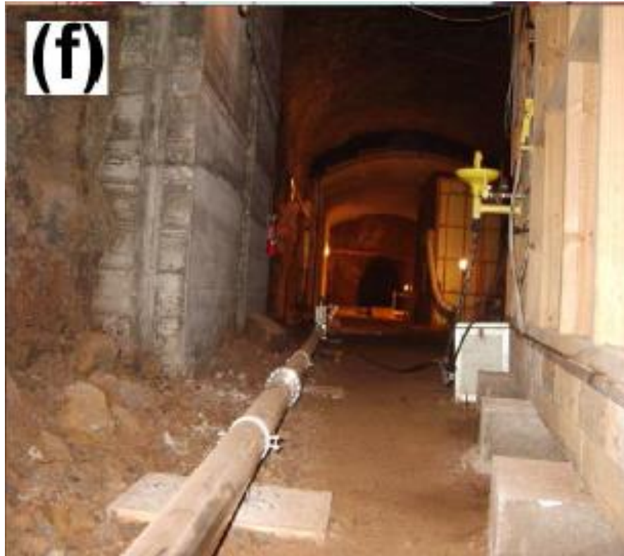
Fig. 2.2. UG-2 ring laser, the largest He-Ne ring laser built underground at the Cashmere Cavern, Christchurch, New Zealand (latitude of -43.575^{\circ} ) which has an area of 834 \text{m}^2 . (Source of the image: [18])
