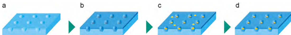
Fig. 1. Concept for improved site-selective quantum dot growth. In the first step a GaAs substrate is pre-structured by lithographic techniques to define nano-holes (a). The native oxide is removed and a thin GaAs buffer layer is grown on top of the pre-structured surface (b). This is followed by InAs QD growth (c). In situ annealing is then used to control the QD distribution and the occupation number of QDs per site (d).
