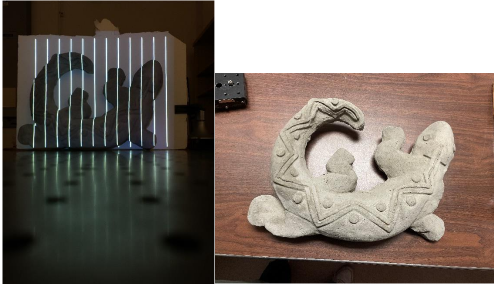
Figure 18. (left) The first image used for triangulation of heavy object using line-shifting method.
