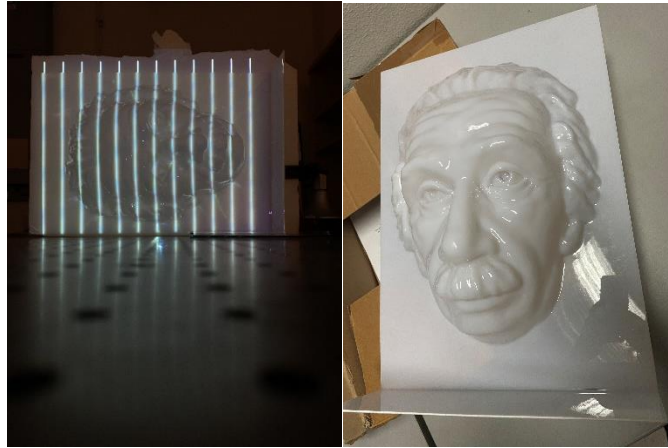
Figure 14. (left) The first image used for triangulation using both line shifting and object shifting methods.
