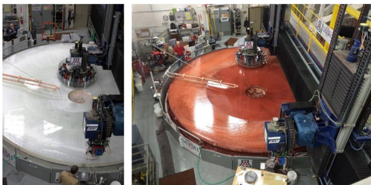
Fig. 3 The LSST primary/tertiary mirror is a coupled optic with an outer diameter of 8.4 m. This coupled design allows for a compact optical layout and powers the extremely wide FOV of the LSST. A 1.2-m stressed lap was used on the tertiary mirror while a 25-cm orbital lap was used on the primary mirror simultaneously using zir-
