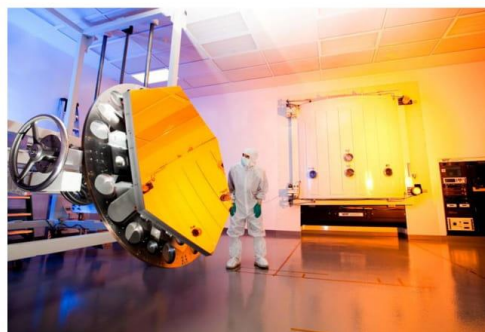
Fig. 14 After precision fabrication of the JWST mirror segments, they require a special coating. Due to the target infrared imaging band, the mirror segments utilize a high uniformity gold coating, which is achieved via vapor deposition. This provides high reflectivity in the imaging bands targeted. Additionally, a protective overcoat layer is applied to help shield the optical surface from damage once deployed [45]
