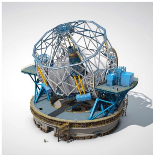
Fig. 6 The E-ELT telescope, the largest of the extremely large NGTs, is a three-mirror anastigmat on-axis design. Nearly 800 individual hexagonal segments will be used to construct the primary mirror, which is 39 m in diameter. The light travels to a suspended convex secondary mirror 30 m above the primary and from there to a concave tertiary mild aspheric mirror. Flat adaptive mirrors guide the light to instruments, located on two Nasmyth structures. Image Credit: ESO
