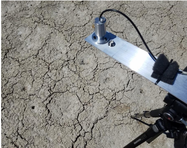
Figure 3.4. Top view of the arm, tripod, and foreoptic of the ASD spectroradiometer. The ground has cracks, holes, and bumps that affect the spatial uniformity of the area. Photo taken 31 Jul 2017.
