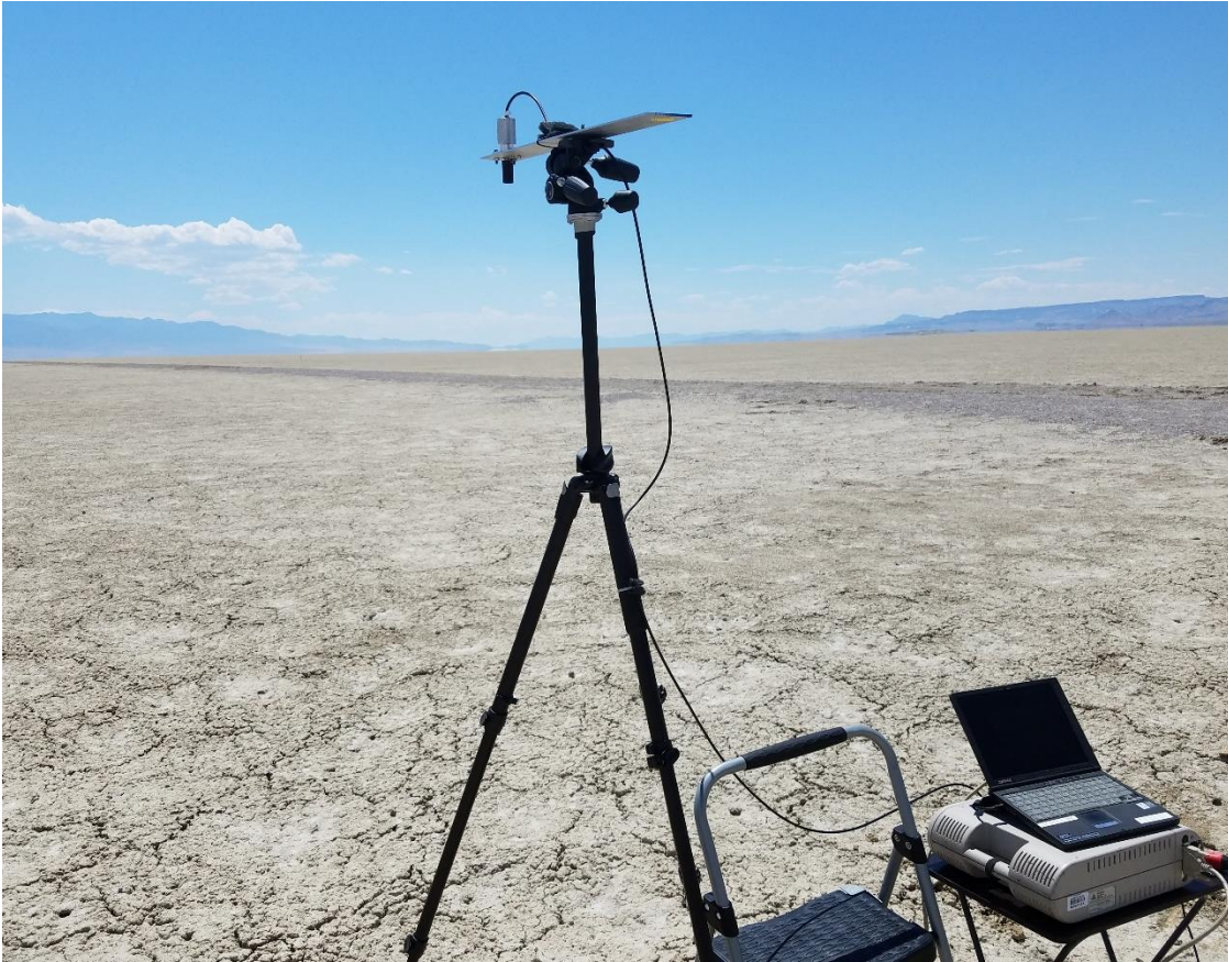
Figure 3.1. ASD setup at Railroad Valley. The foreoptic is mounted on the aluminum arm on the tripod. The signal electronics are on the table under the laptop and the laptop stored the data taken. Fiber optic runs from the foreoptic to the electronics.
