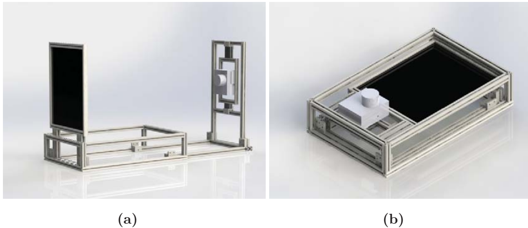
Figure 2.8: The second portable DR system, showing (a): the DR system in imaging mode, (b): the system collapsed.
