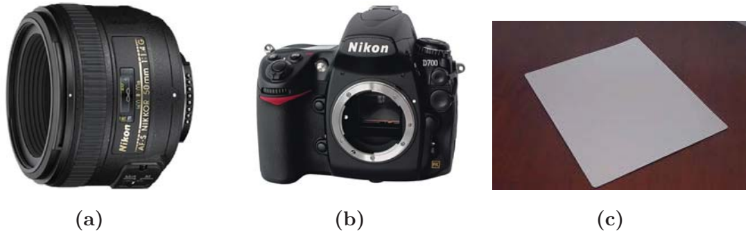
Figure 2.4: The imaging components that were used in the DR system, (a): Nikkor lens, (b): Nikon D700 camera, and (c): phosphor screen.
