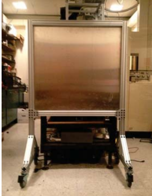
Figure 2.11: The lead shield for stopping direct x-rays.
