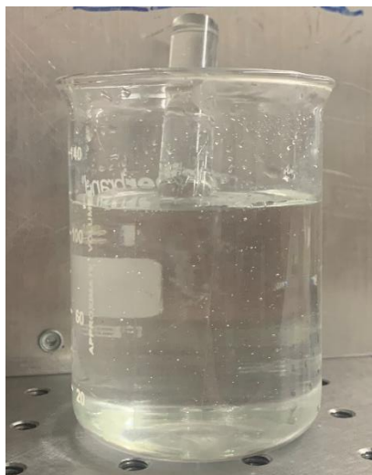
Figure 2 Borofloat Rod Partially Submerged in Index Matched Glycerol
