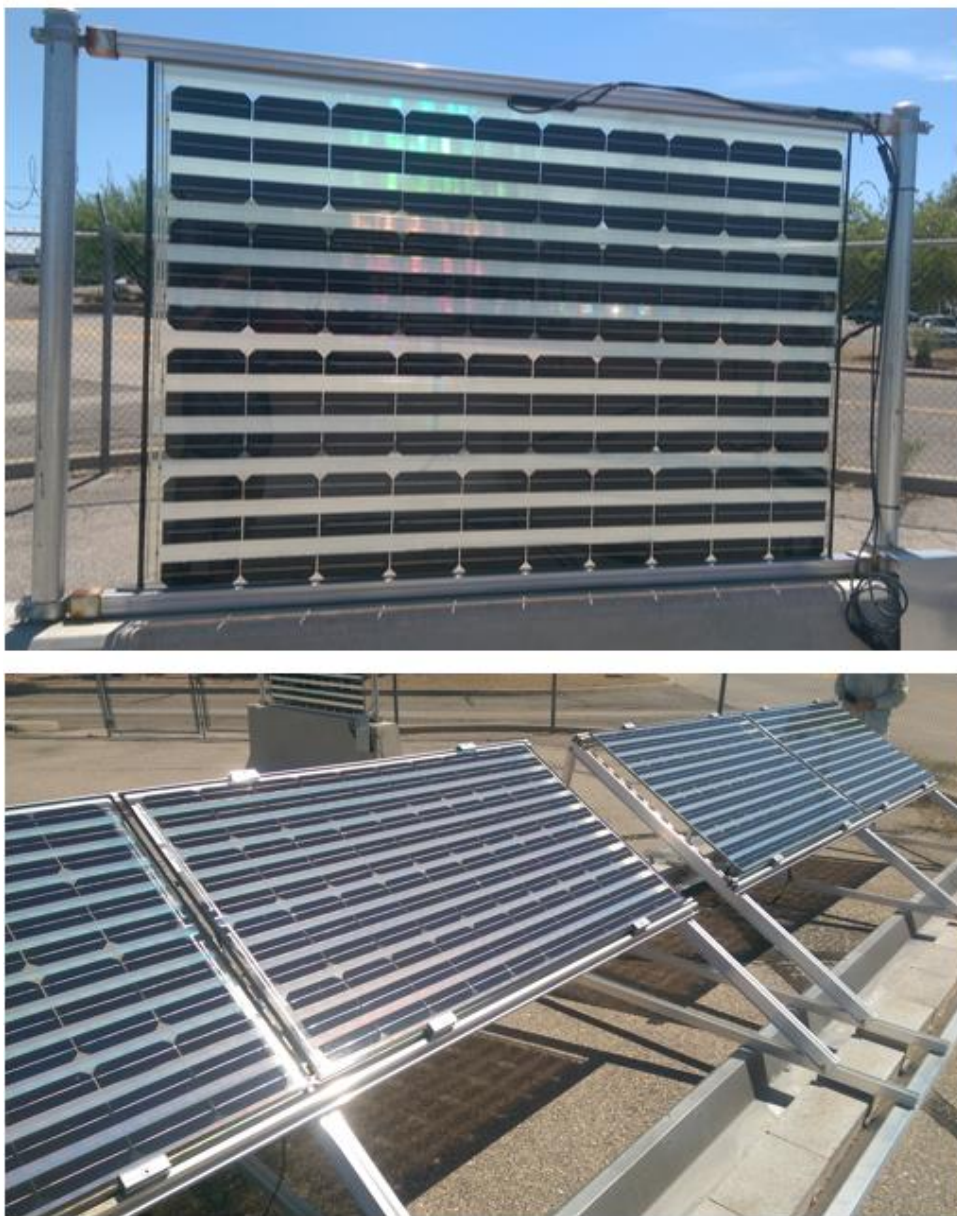
Figure 6.1: Holographic solar concentrator modules made by Prism Solar that use dichromated gelatin holographic material.
