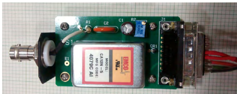
Figure 4.3: Picture of a programmable high-voltage unit used on AdaptiSPECT. The wiring on this unit is (from bottom to top): 5V ground, DAQ ground, DAQ command, 5V reference, input V.
