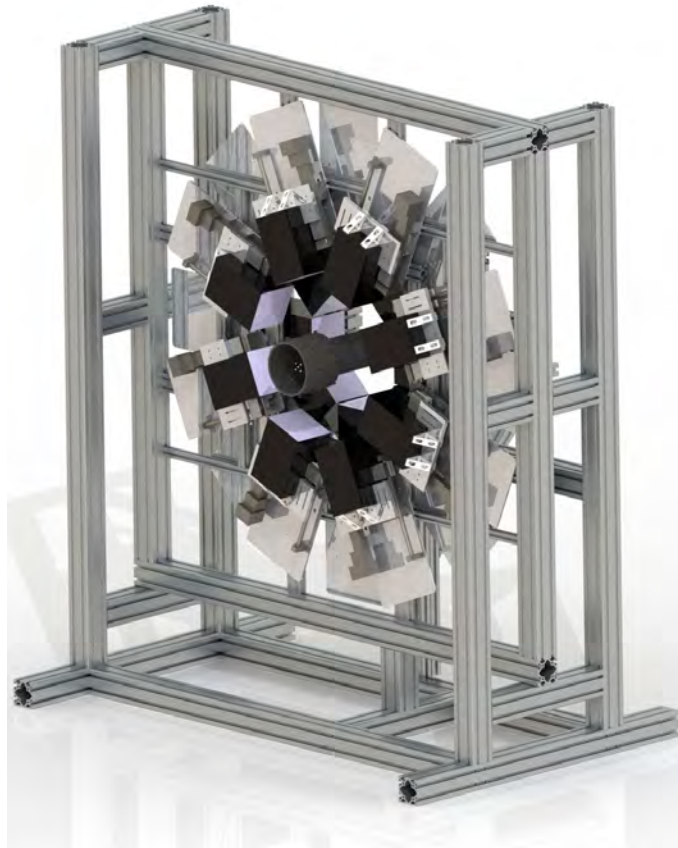
Figure 2.18: Solidworks TM rendering of the AdaptiSPECT gantry. The front ring of 8 detectors is visible. The translation stages which allow the radial translation of each detector are also visible.
