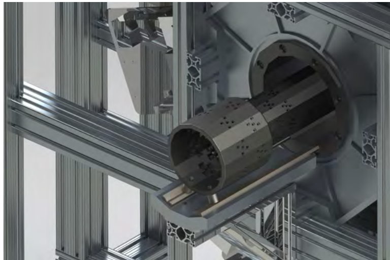
(b) CAD rendering of the aperture support and motion system on the low-magnification ring segment side.
