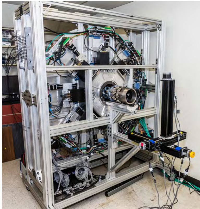
Figure 4.13: Complete AdaptiSPECT system. Photo courtesy Joseph Ortiz.
