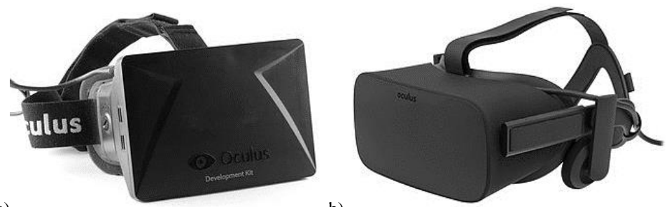
a) b) Figure 6. a) Oculus' 2012 Development Kit 1 (DK1) [23] b) Oculus Rift (2016) Consumer Version 1 (CV1) [24].
