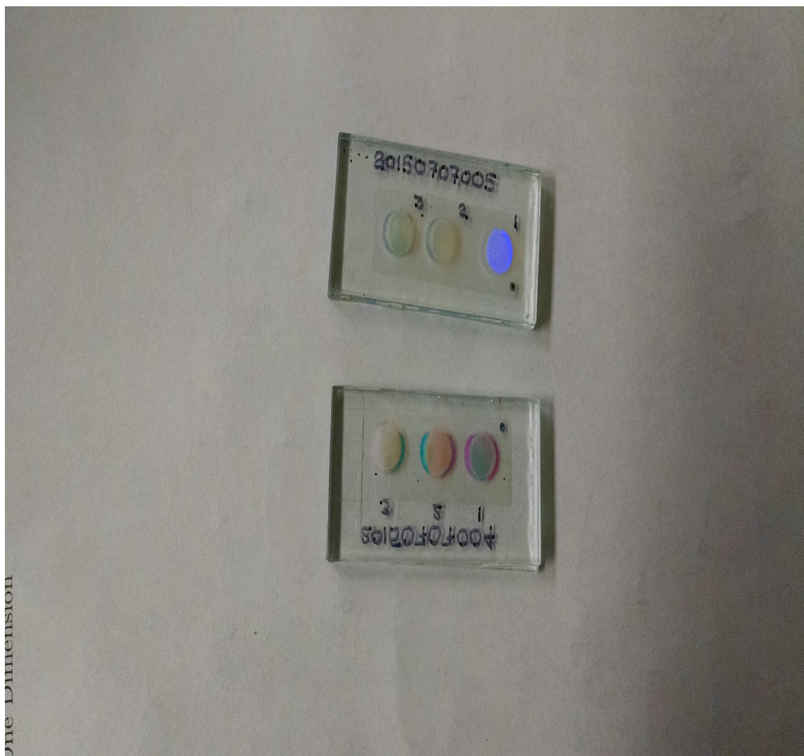
Figure 4.2: Picture of our first prototypes of the volume hologram, written at RL Associates.
