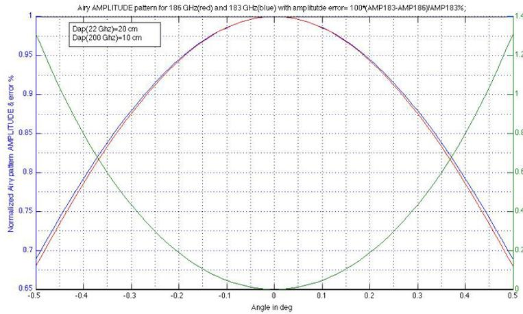
Figure V.5.4: .Normalized gain at 183 & 186 GHz and residual amplitude error of 0.3% at 0.25deg when the ratio of the received amplitudes is formed for lens diameters of 10 cm
