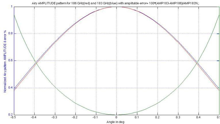
Figure V.5.2: Normalized gain at 183 & 186 GHz and residual amplitude error in % when the ratio of the received amplitudes is formed for lens diameter of  $D_{\text{lens}}=30$  cm ( only 15 cm of the diameter is illuminated) Maximum amplitude error  $\sim 0.8\%$  at 0.25 deg pointing error.
