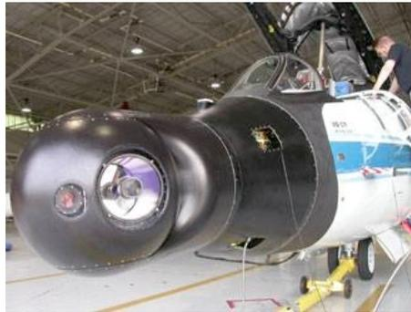
Figure I.7.1: The WAVE system mounted on the nose of a WB-57F. ATOMMS will replace the optical telescope in this system. A microwave transparent radome will replace the front skin and optical window.
